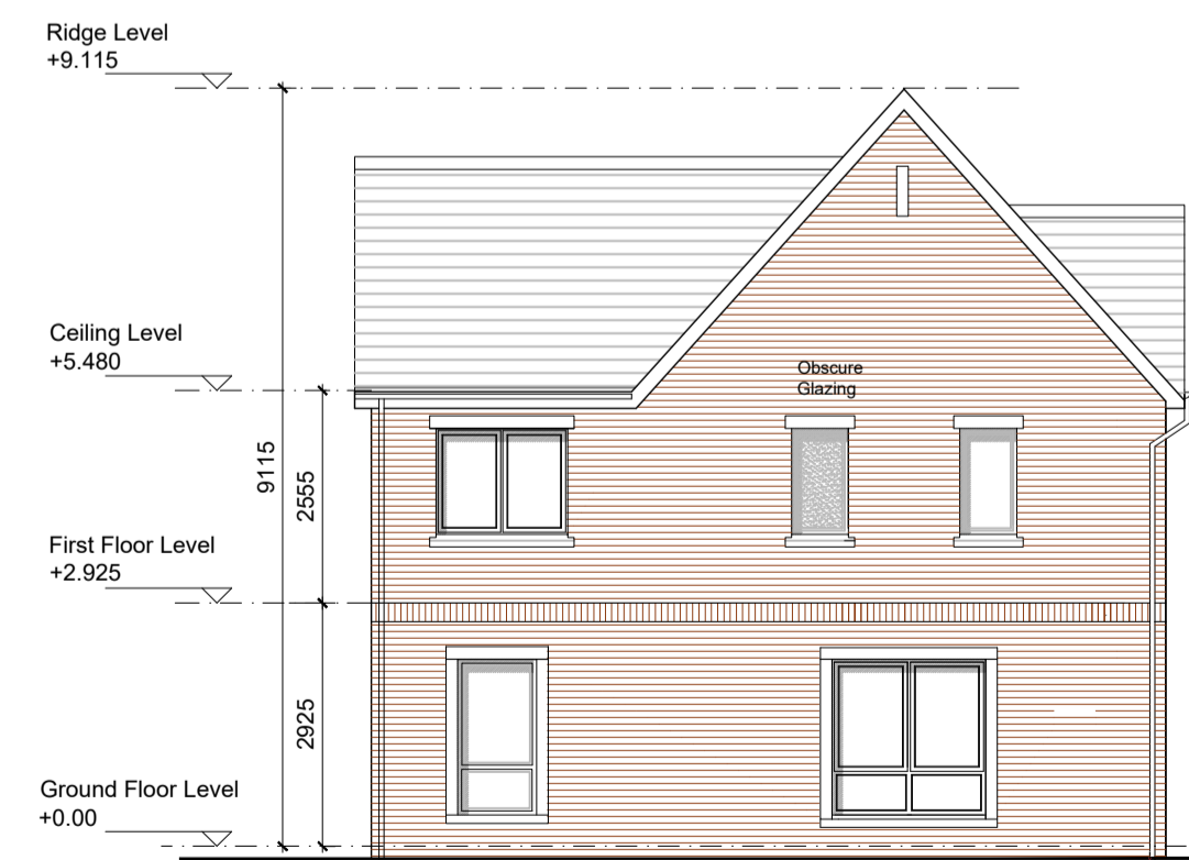
SIDE ELEVATION (Type D) Scale 1:100 Mirrored where applicable
